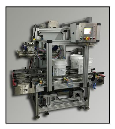
ABA-M385 is a two head net weight filling machine which was designed to fill on alternating lanes. This was done in order to achieve a continuous flow of a high viscosity extruded product. The system functions such that it fills on one lane while an empty container is being conveyed into position on the 2<sup>nd</sup> lane. Once the first container is done and begins to move out of the fill area, filling immediately begins on the 2<sup>nd</sup> lane.
