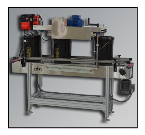
ABA-PRESS-5GALL-P is a powered 5 gallon lid press which is designed to pull containers through while simultaneously pressing lids on. This press works in conjunction with a powered conveyor.
