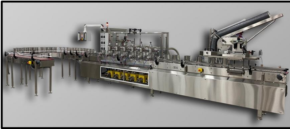
ABA-M496 is a top fill machine featuring a horseshoe conveyor, lid dropper with downstacker, roller lid press, and one gallon pumps. https://youtu.be/5urGrNhoz7A
