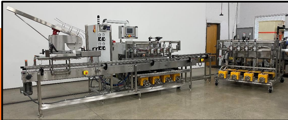
ABA-M527 is a 4 head, volumetric, push across (Z-frame) filling machine for metal and plastic gallon cans. It features a roller lid press and lid dropper with downstacker as well as two fill carts. https://youtu.be/PHSMg6appwc
