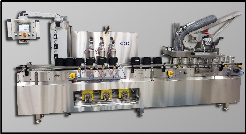
ABA-M527 is a 4 head, volumetric, push across (Z-frame) filling machine for metal and plastic gallon cans. It features a roller lid press and lid dropper with downstacker as well as two fill carts. https://youtu.be/PHSMg6appwc
